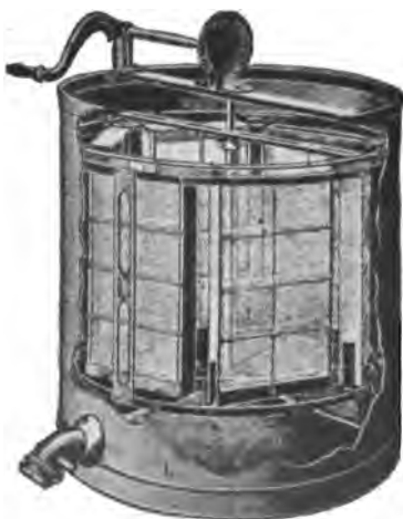
FIG. 22.—Automatic reversible honey extractor. (By permission U. S. Dept. Agric.)
